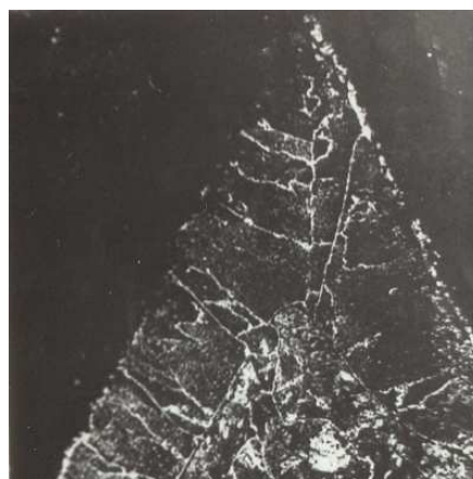
Figure 20. Microstructure of prong of Xu-Tec HSS saw blade.
