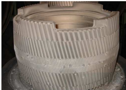
Figure 22. Colloid mill after Xu-Tec plasma surface alloying, carburizing and quenching and tempering.
